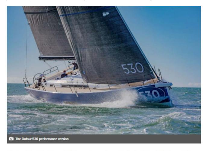
Like her sisters in the former "Performance" range, her mainsail sheet is located in the cockpit, more winches, hydraulic backstays and boom vang. She also comes with upgraded mast and boom for an increased sail area of 20 m2. and her 2.80-metre keel comes complete with a lead bulb.
